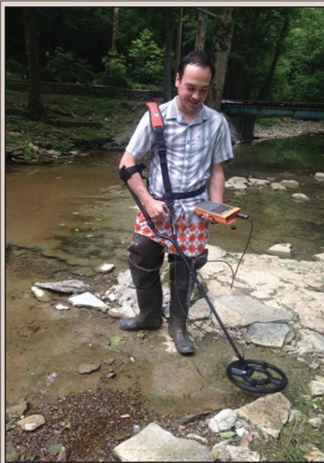
FIG. 1. Passive Integrated Transponder (PIT) tag telemetry was used to detect Queensnakes ( Regina septemvittata ) in Jessamine County, Kentucky (USA). Telemetry involved the use of the Biomark HPR Plus portable reader (orange) and BP Portable Antenna.
